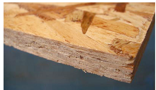
Photograph 4: Oriented Strand Board “Take 2” —Finished product – an engineered “structural use panel.”
