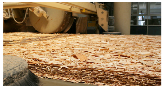
Photograph 3: Oriented Strand Board “Take 1” —Note the layered mats of aligned strands prior to heat and pressure.
