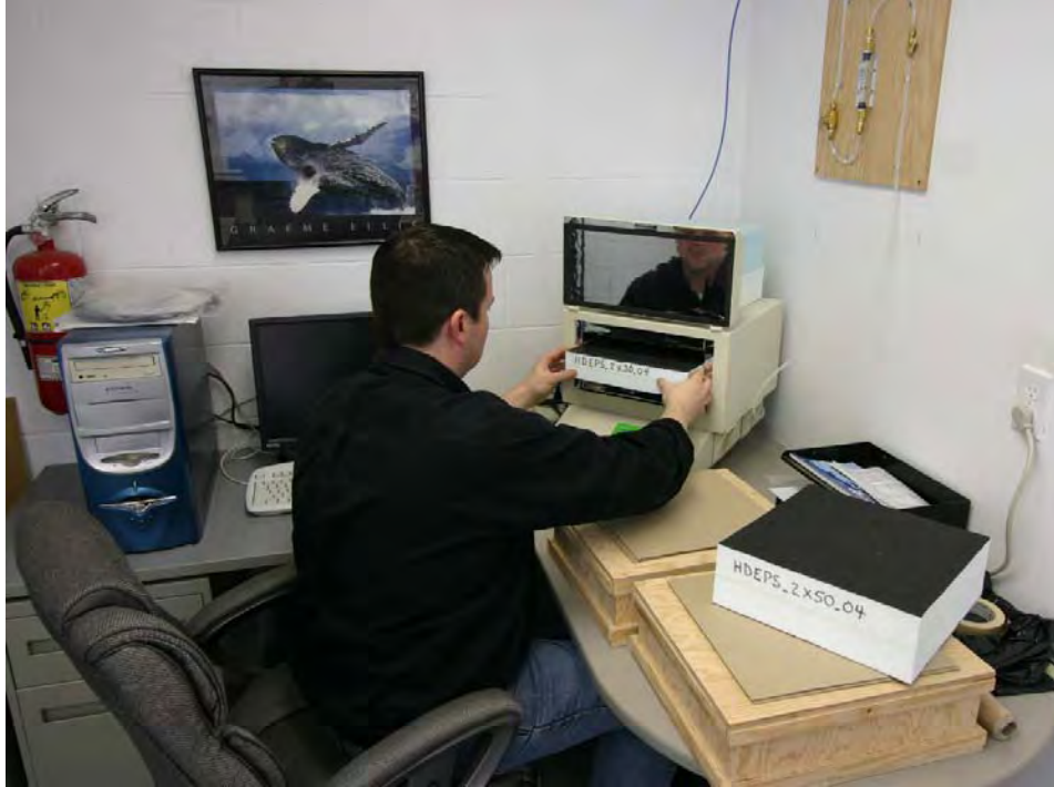
Figure 33 – Testing Calibration Panel Specimens in BSC’s 514 Test Machine
