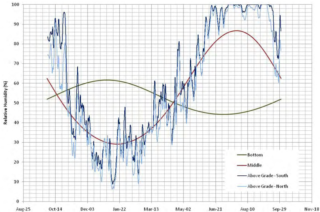
Figure 13 : Predicted Relative Humidity at the Surface of the Polyethylene Vapor Barrier for Case 3
