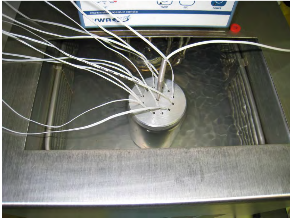
Figure 18 - Temperature Sensor Calibration Setup
