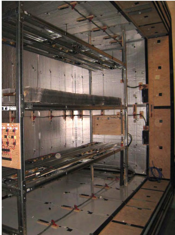
Figure 3 – Upper & Lower Heating Arrays & Cooling Coil in Meter Box
