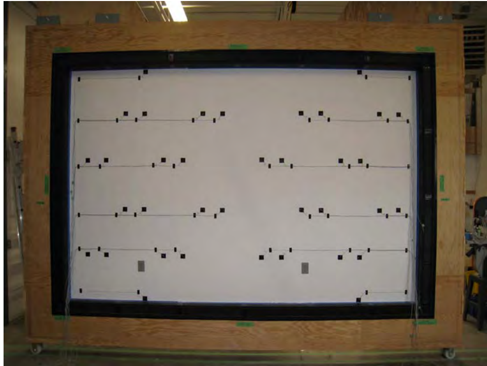
Figure 7 – Wall Cartridge with Test Wall Specimen Installed & Instrumented for Testing
