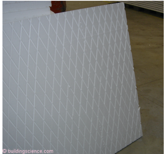
Photograph 3: Expanded Polystyrene Draining Insulation - After a couple of years we got grooved rigid expanded polystyrene (EPS). It was a 60's thing...it was “groovy” ... The “groovy” side would face the waterproofing. The non “groovy” side would face the dirt.
