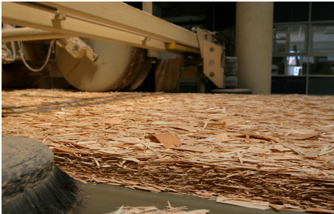
Photograph 1: Oriented Strand Board – take a fast growing “teenager” tree and flake it, add the Colonel’s eleven secret herbs and spices, smooch it together under heat and pressure and coat it with “water stay away stuff”. (c) Matthias Kabel from the Wikipedia Commons; https://en.wikipedia.org/wiki/Oriented_strand_board#/media/File:OSB_production.jpg
