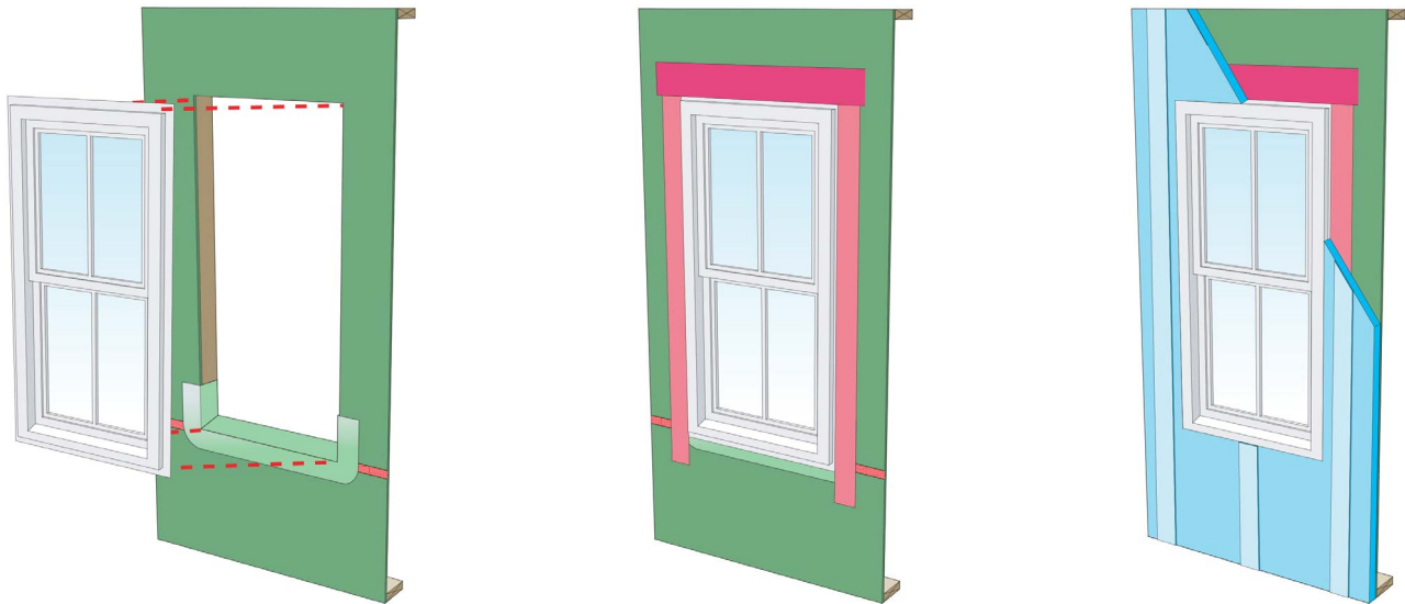
Figure 2a – Window Installation: Note the “pan flashing” at the bottom of the rough opening and note that the window flange is installed directly on the OSB sheathing. Figure 2b – Window Installation: Flashing tape is used to provide water control layer continuity and air control layer continuity. Figure 2c – Window Installation: Continuous insulation is installed over the OSB sheathing. Note that the water control layer is behind the continuous insulation.
