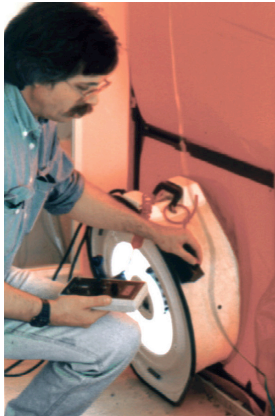
Photograph 1: The Ubiquitous Blower Door —I love what it can do and hate what it can't do even though people say that it can. That is pretty clear, isn't it?
