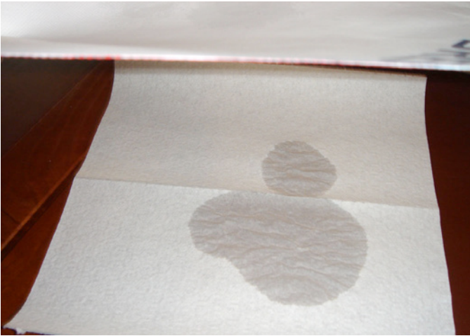
Photograph 13 – Wet Spot: Failure is pretty dramatic when it happens. It should fail in less than 60 minutes if it is going to fail. The water solution just stays there for a long while and nothing happens. Then, all of a sudden, it goes through. More exciting than watching paint dry.
