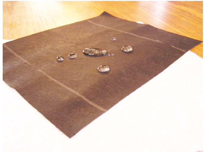
Photograph 3 (top left) – Wet Siding: Water that used to drain and not be absorbed now passes through the field of the building paper and is absorbed. More water is now retained for a longer period of time. Photograph 4 (top right) - Tar Paper Test: A teaspoon of water is placed on tar paper placed over a paper towel. Look at how the water beads up on the surface. A beautiful sight.
