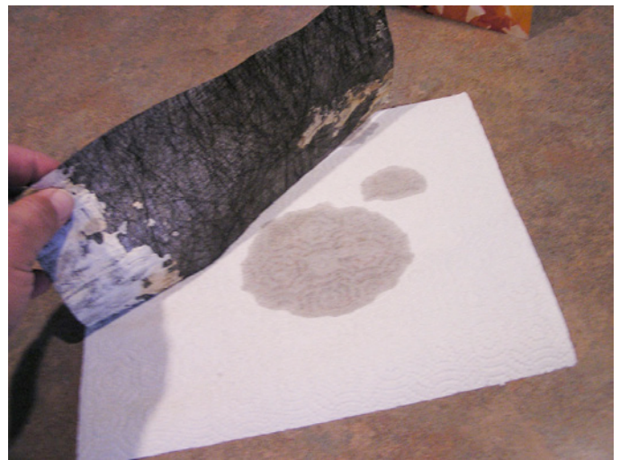
Photograph 5 (above left) – No Wet Spot: If the water beads up and does not wet the paper towel – it passes Joe Test 1. Photograph 6 (above right) – Nice House Gone Bad Stuff: In the case of the house we were looking at, the sample product removed from the wall failed Joe Test 1. Most products pass Joe Test 1 before they are installed. But all products that fail in the field seem to fail Joe Test 1.
