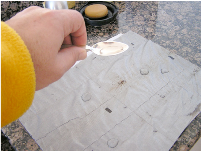
Photograph 10 – Wood Sugars and Tannins: I began to notice that when I held failed housewraps up to the light they were darker in some spots than others. They would fail Joe Test 1 in the dark stained areas and pass Joe Test 1 in the non-dark areas. It became very obvious with lighter colored housewraps. What caused the discoloration? That part was easy. Wood sugars and tannins. Water-soluble extractives. “Weak” surfactants by another name.
