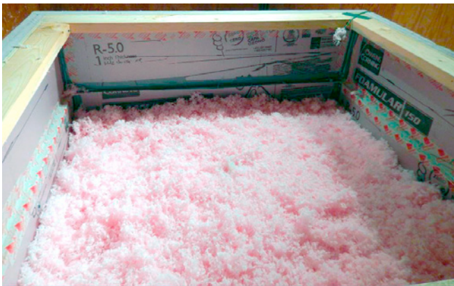
Photograph 6: Buried Duct Laboratory Test Continued – Loose fill insulation “burying” the ductboard ductwork test box.
