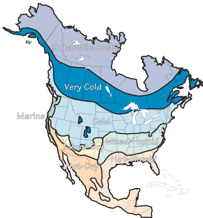
Figure 3: Hygrothermal Regions —Note that IECC Climate Zones 7 and 8 are considered “very cold” and “subarctic/arctic”.
