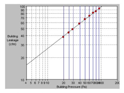
Typically, depressurization leakage amounts were smaller than pressurization leaks, but only by a small margin. This can be attributed to the fact that a depressurized cabinet would tend to draw loose-fitting parts tighter.
