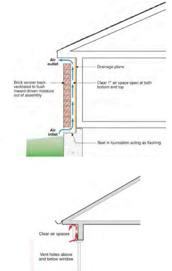
To effectively uncouple a reservoir cladding from a wall system by using back ventilation, a clear cavity must be provided along with both air inlets at the top and bottom of each wall section.
