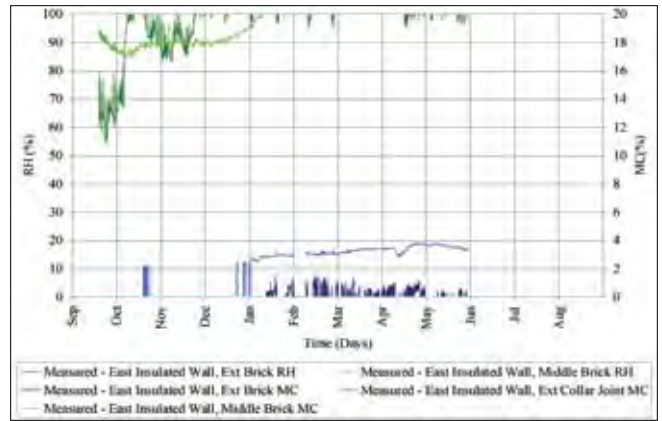
Figure 6. Measured RH and MC in east insulated wall. Actual relative humidity and moisture content (wood wafer) measured in the insulated east wall. The moisture content is well below thresholds for freeze-thaw. MC values shown are for the wood resistance sensors embedded in the brick, instead of the corresponding brick moisture content in order to increase measurement resolution.
