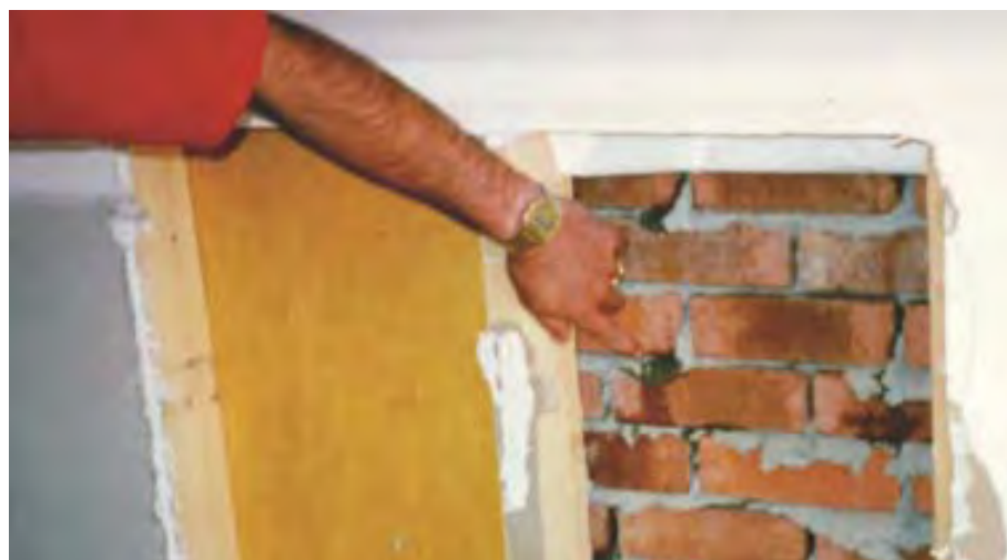
Figure 1. In this hose test, water penetrated brick veneer in less than a minute (below). The wall behind brick veneer must be designed to drain.
