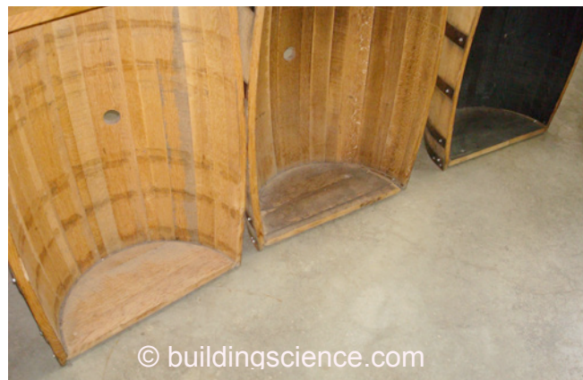
Photograph 2: Charring of Barrels —Un-charred, medium charred, heavily charred barrels. The charring leads to distinctive flavors as the “clear liquid spirit” changes its color due to the charring to a deep amber color and changes its taste and smell into a uniquely American experience.
