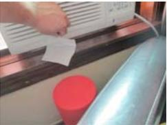
*Measurable air leakage at window AC units*
