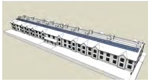
South Roof with Photovoltaic Array Taft Hill Manor, Uxbridge, MA
