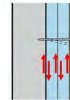
Vertical movement resistance provided by friction between layers
