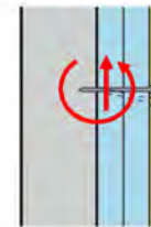
Shear and rotational resistance provided by fastener to wood connections
