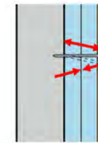
Rotational resistance provided by tension in fastener and compression of the insulation
