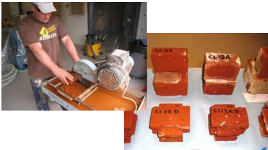
Freeze-Thaw Resistance of Clay Brick 2010.12.06
