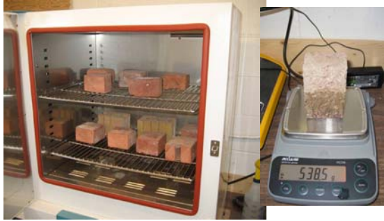
Freeze-Thaw Resistance of Clay Brick 2010.12.06
