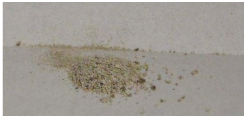
Dried mineral precipitate from inlet strainer
