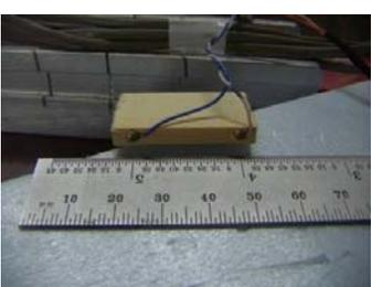
A close-up photograph of the yellow wafer sensor with a ruler for scale. The sensor is a small, rectangular, yellow device with a blue wire.
