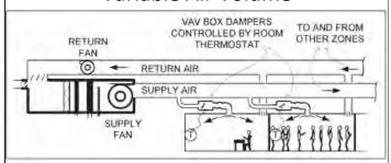
Poor IAQ: ventilation controlled by thermostat
