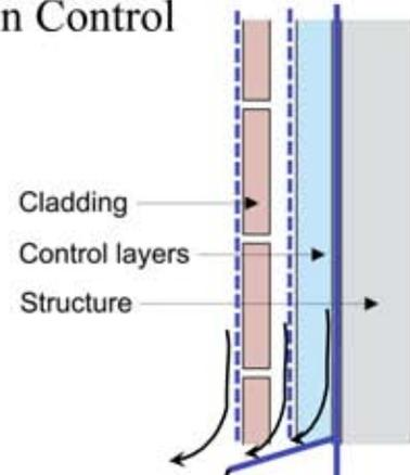
The diagram shows a cross-section of a building wall assembly. From left to right, it consists of cladding (represented by three stacked rectangular blocks), control layers (a vertical blue line), and the structure (a grey block). A blue arrow indicates rain falling from the top left, hitting the cladding. A dashed blue line shows the path of water being directed down and away from the control layers. Labels with arrows point to 'Cladding', 'Control layers', and 'Structure'.
