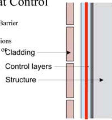
The diagram shows a cross-section of a building wall assembly. From left to right, it consists of cladding (represented by three stacked rectangular blocks), control layers (a vertical blue line), and the structure (a grey block). A solid red vertical line runs through the control layers, representing the thermal barrier. Labels with arrows point to 'Cladding', 'Control layers', and 'Structure'.
