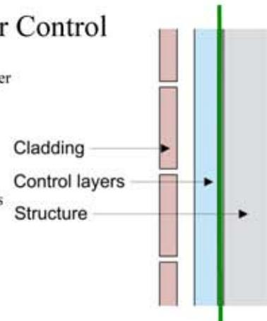
The diagram shows a cross-section of a building wall assembly. From left to right, it consists of cladding (represented by three stacked rectangular blocks), control layers (a vertical blue line), and the structure (a grey block). A solid green vertical line runs through the control layers, representing the air barrier. Labels with arrows point to 'Cladding', 'Control layers', and 'Structure'.
