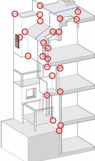
A 3D cutaway diagram of a building's structural frame, showing multiple levels of floors and columns. Red circles are placed at various points where different materials, planes, or trades meet, indicating locations where detailed design is required. The diagram is labeled 'Building Science.com' and '31/175'.
