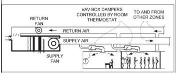
Poor IAQ: ventilation controlled by thermostat
